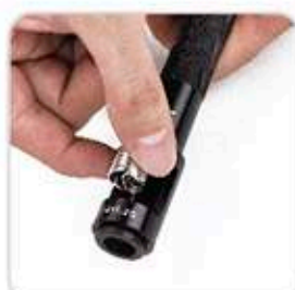
3. Load coiled insert into Coil Shielding Collar
