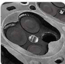
6. Thread is repaired and ready to use
