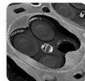
6. Thread is repaired and ready to use
