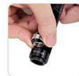
3. Load coiled insert into Coil Shielding Collar
