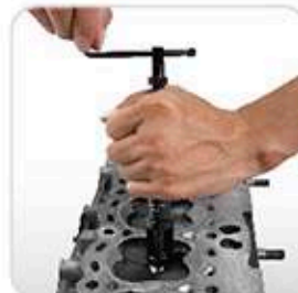
4. Screw coil into thread slowly
