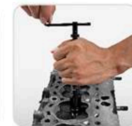
4. Screw coil into thread slowly
